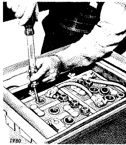
Figure 20-5-2—Checking Specific Gravity of Battery with a Hydrometer
