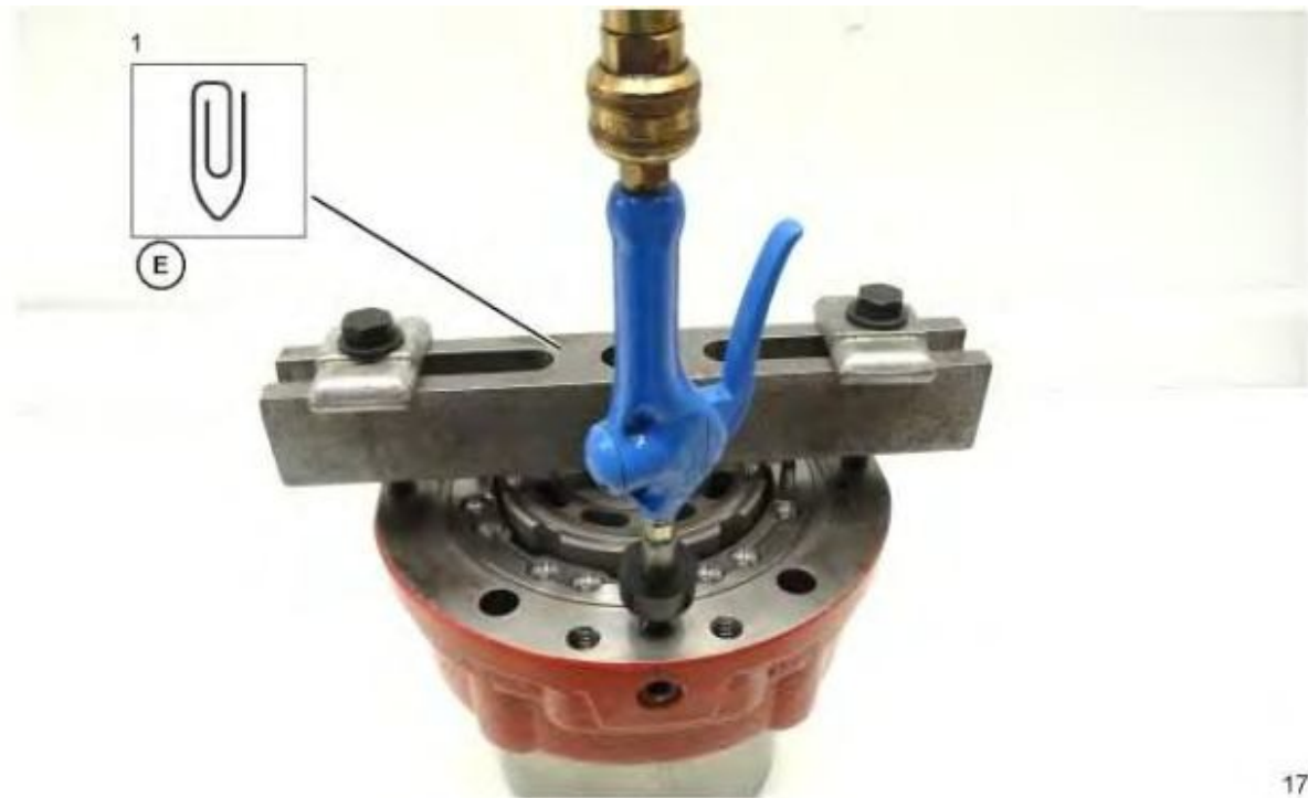
Illustration 17 Use air pressure to unseat the brake piston.
